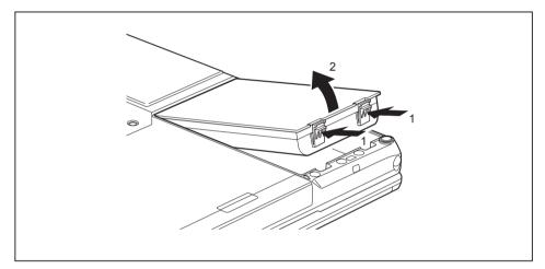
Press in the two catches (1), keep them pressed and lift the battery out of the battery compartment (2).
